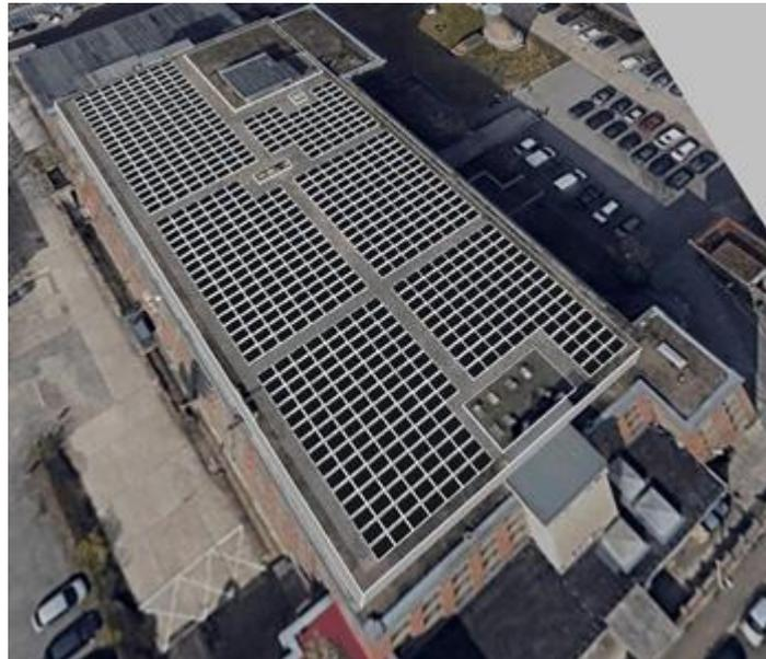
Fig. 12: Simulated PV-Plant geometry for building 18
