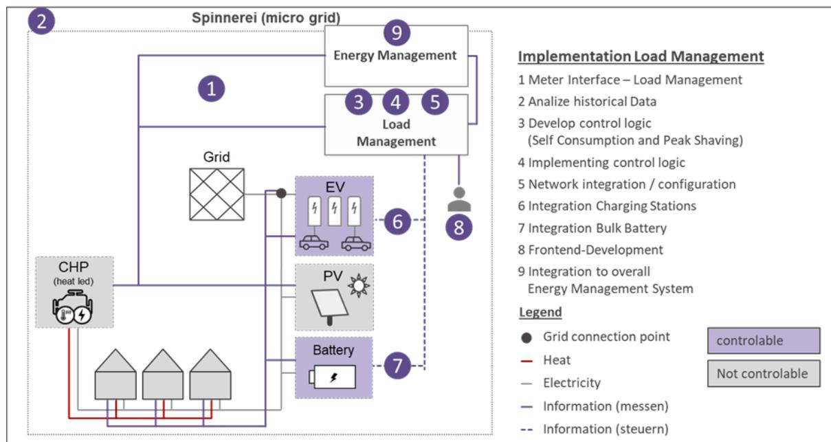
Figure 12: Architectural design to implement bidirectional charging (Source: CEN)
