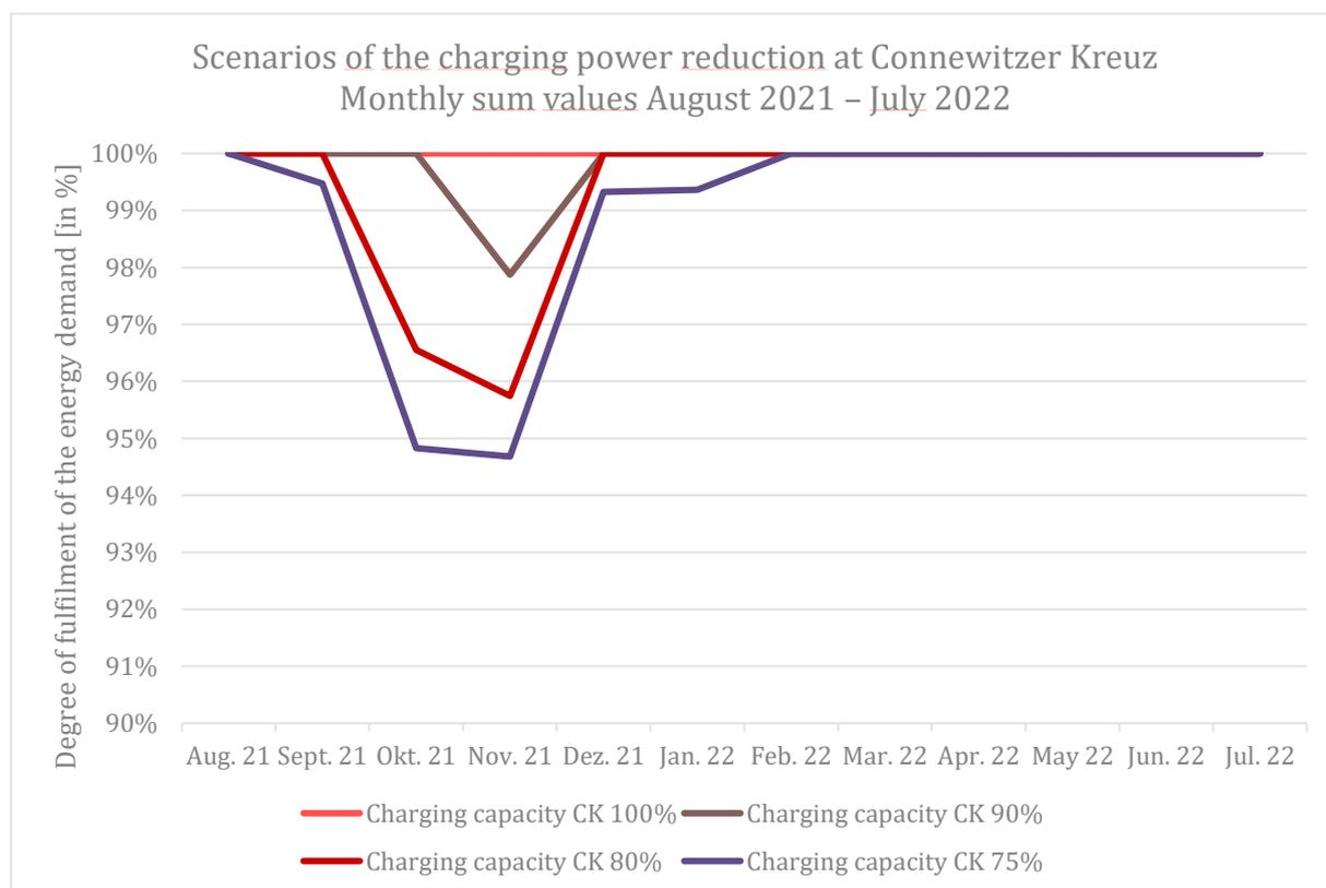
Figure 9: Scenarios of charging power reduction at Connewitzer Kreuz (Source: FHG)
