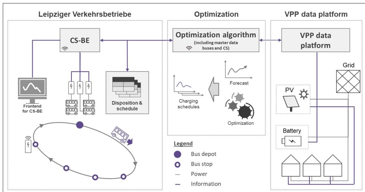
Figure 10: Load management in the bus depot (Source: FHG)
