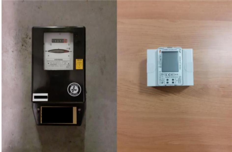
Figure 16: Old electricity meter and new remotely readable meter (Source: CEN)
